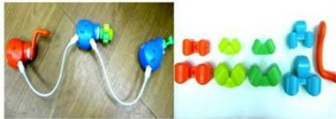
Figure 3: Actives (left) and passives (right) in Topobo system
