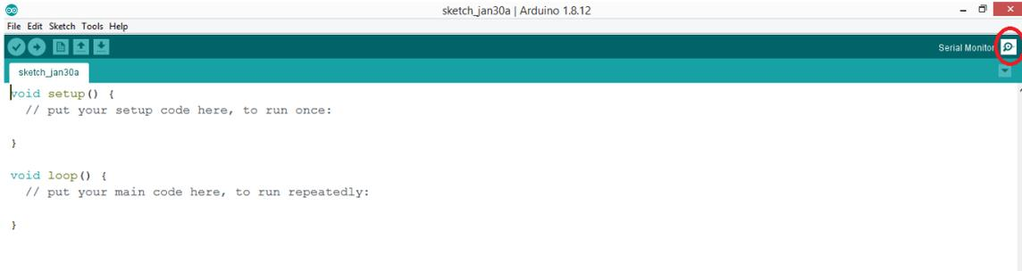
**Figure 3:** Arduino IDE window. Click the Serial Monitor Icon to open the Serial Monitor.
