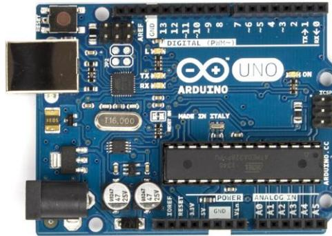
**Figure 1:** The Arduino UNO board.
